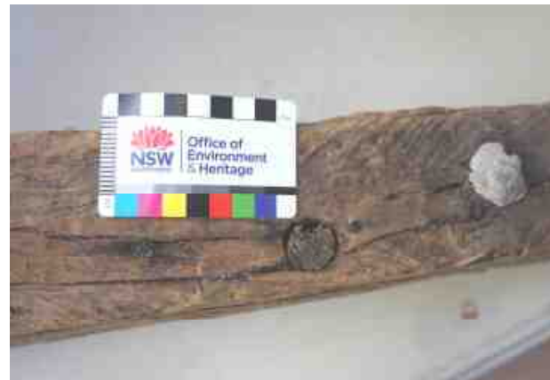
Part of a ship's rib showing a trunnel and lead-covered nail. A piece of this timber has been sent for analysis to confirm its species. (Photo Brad Duncan)
