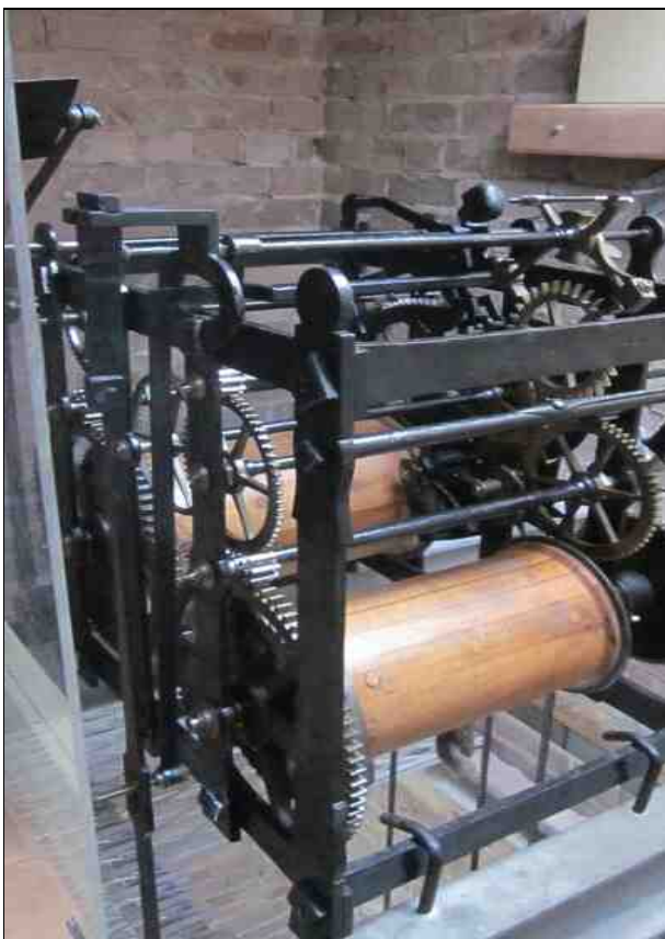
The pendulum side of the clock showing the weight barrels now redundant due to the electric winding mechanism. The rod on the goes down through the steel mesh floor .
