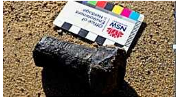
A short iron bolt – 25mm diameter with a hex head. The fine thread continuing almost to the head suggests a bolt from machinery not a timber fastening.
