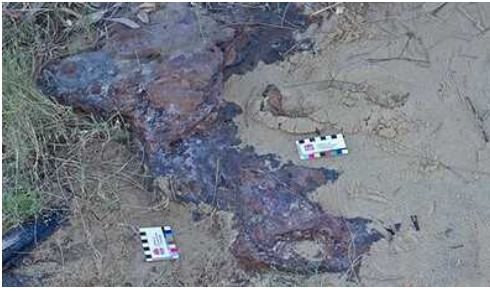
These images show three of the six, irregularly bent pieces of 7mm iron plate that were found. (photos: D. Forbes)
