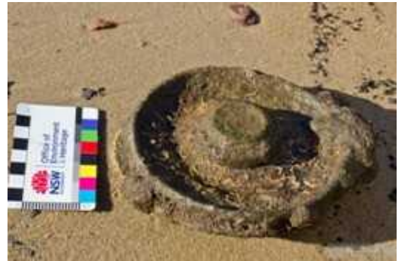
Here is an iron pulley for a V belt drive and a shaft of approximately 30mm that has been sawn or broken off.
