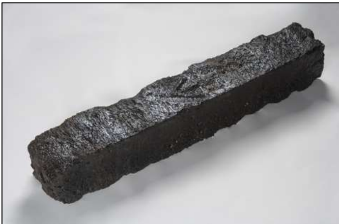
Image 1: A piece of Endeavour's iron ballast (or kentledge) from HMB Endeavour recovered in 1969 from the Barrier Reef and now in SSHS Museum. Note the broad arrow denoting government ownership. [Image from the ANMM website 2 : object number 00029143, weight 85 kg]
